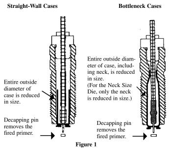
The entire cartridge case enters these dies, flush to the shellholders.
